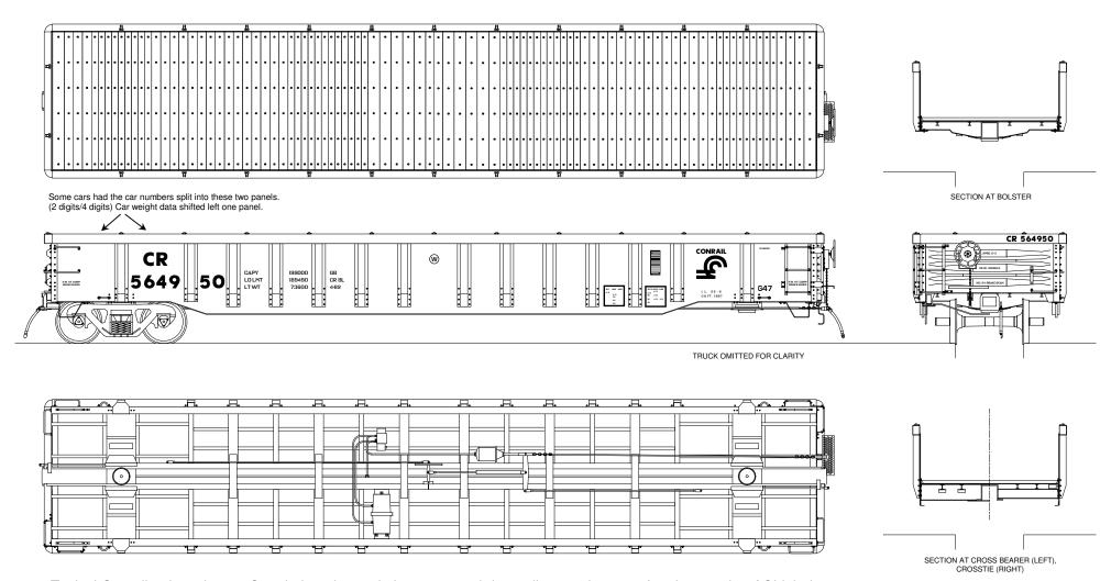
Typical Conrail paint scheme. Certain lettering variations occurred depending on shops performing repaint. ACI labels not applied to cars repainted after 1978. 2 panel lube plates replaced by single consolidated stencil in the mid 80's.
